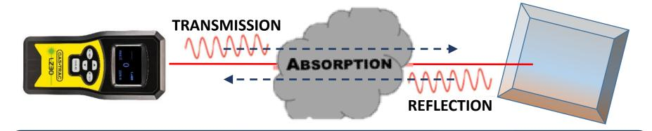
Methane (or any gas) absorbs a specific wavelength of light
